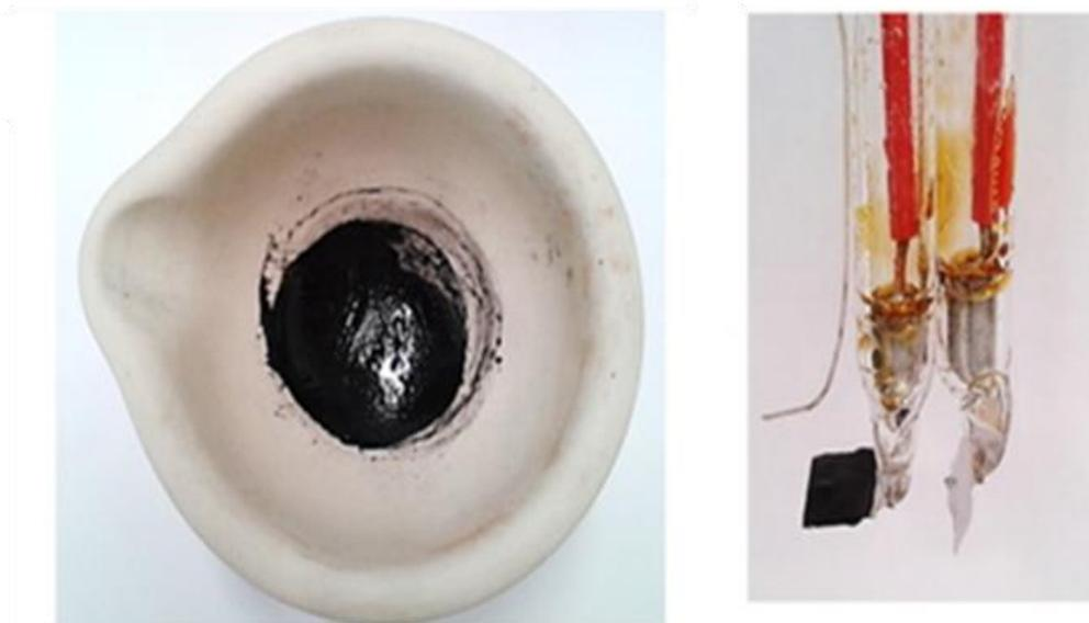
*Figure 2.6: Paint casting method paste obtained from the mixing of powder of mineral or metal compound with a DES (left) and WE bended at 90 °C holding the paste (right).<sup>23</sup>*
