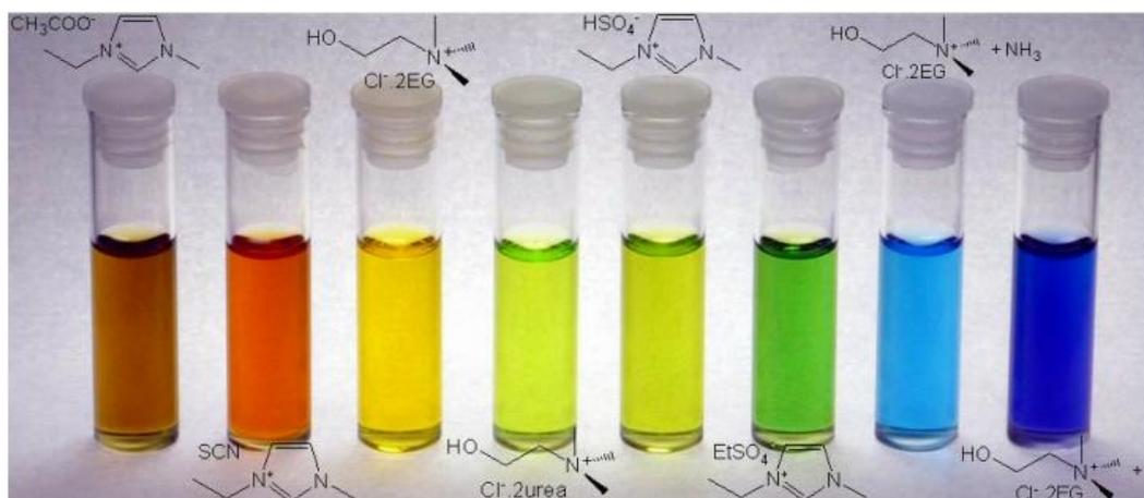
*Figure 1.12: Colored solutions of  $\text{CuCl}_2 \cdot 2\text{H}_2\text{O}$  dissolved in different ILs and deep eutectic solvents.<sup>105</sup>*
