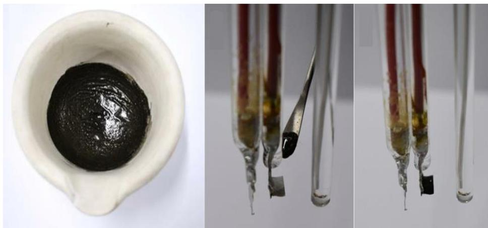
*Figure 4.2: Setup of the paint casting method. Paste of solid material mixed with EG:ChCl (left) and three electrode system with the paste painted on the working electrode (right)*
