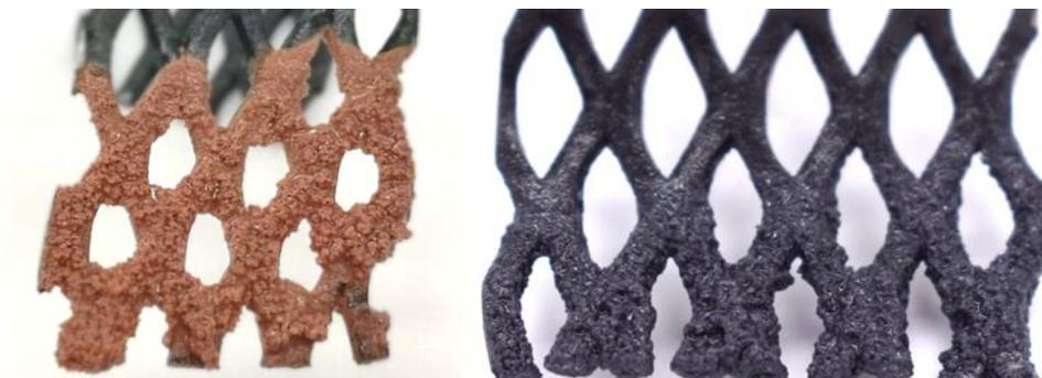
Figure 7.14: Deposits on WE after electrochemical dissolution of Cu<sub>2</sub>O (left) and PbO (right) in EG:ChCl.
