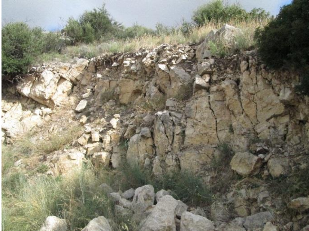
Figure 2.7. Scillato Formation is highly fractured, with fractures varying in aperture from few centimetres up to 15-20 cm. Not available scale for this picture.
