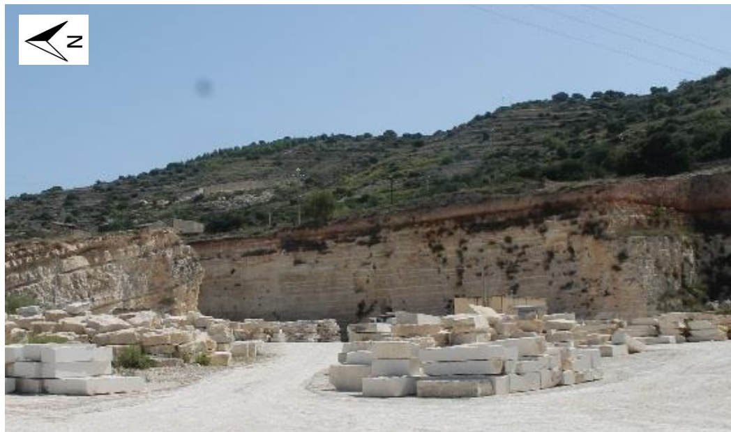
Figure 2.8. The Comiso quarry. It is possible to note the sequence of monotonic layers of limestone dipping gently towards North.
