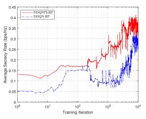
Fig. 9. Average secrecy rate with delay constrained vs. training iterations in *Case 2*.
