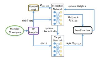
Fig. 3. The structure of training neural networks in DDQN based scheme.
