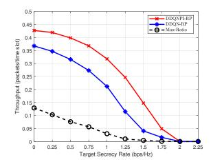
Fig. 7. The comparison of throughput between proposed schemes and Max-Ratio scheme for *Case 1* with different secrecy target rate.
