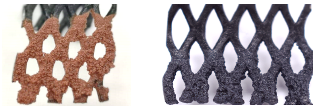
Figure 3: Material deposited on the cathode after electrochemical dissolution of Cu 2 O (left) and PbO (right) in EG:ChCl.
