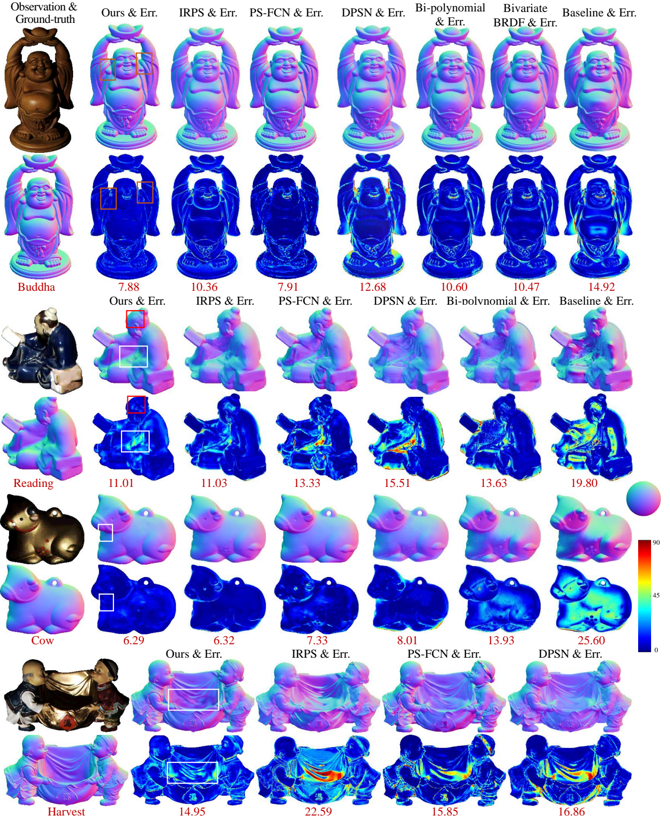
Fig. 6. Quantitative results for strong non-Lambertian real-world scenes from the DiLiGenT benchmark dataset. Err. is short for error map. The numbers under the error maps represent MAE in degrees. The contrast of observations are adjusted for easy view. The red boxes are regions with specularities, the white boxes are the regions with cast shadows, and the orange boxes represent the region with non-convex surfaces (crinkles). Our method produces more accurate estimations in those regions compared with the other methods.
